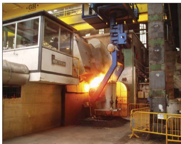
Fig. 19 : A large capacity crane mounted ladle.
