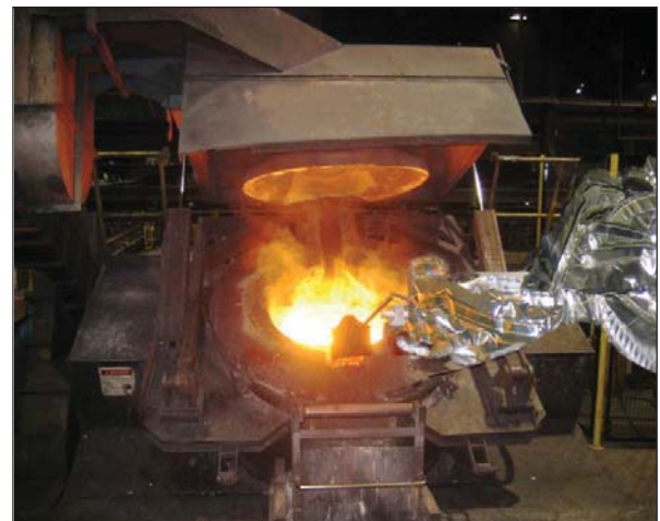
Fig. 18: A robot being used to remove slag.
