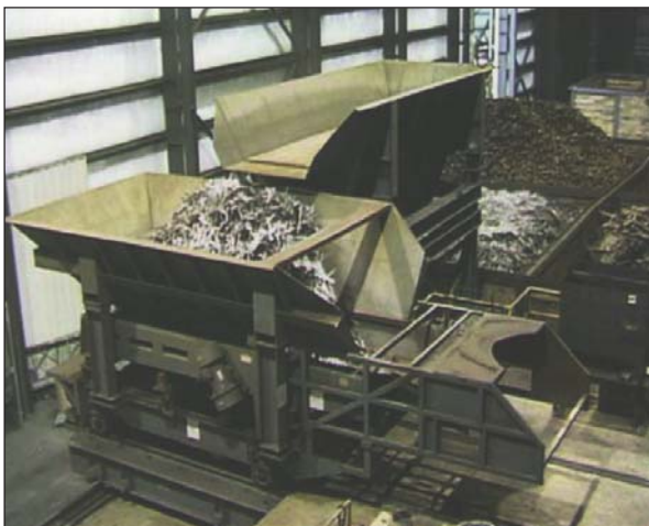
Fig. 4: Feeder and weigh hopper.
