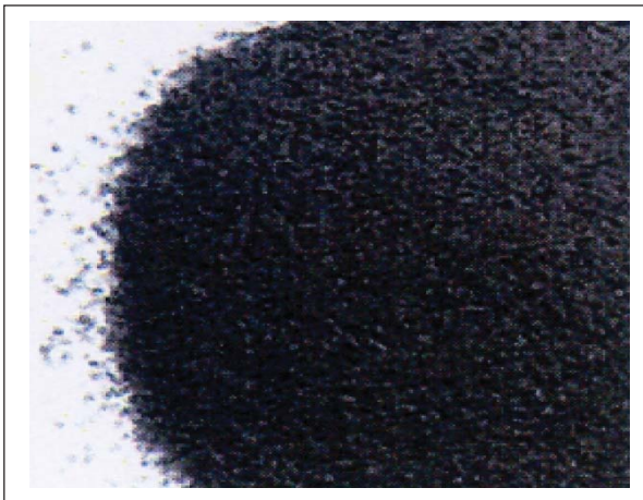
Fig. 17 : Correctly sized “trim” graphite.
