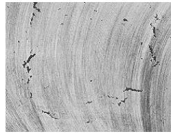
Gas inside metal section
