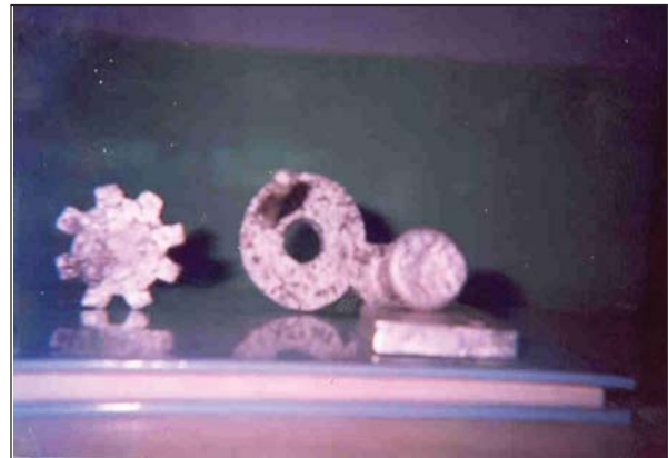
Fig. 3 : Samples made by magnetic moulding.
