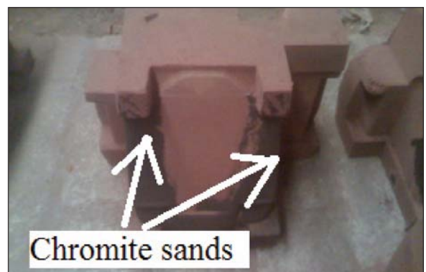
Fig. 12: Chromite sands to prevent hot tears.
