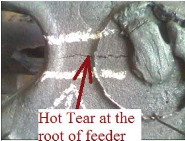
Fig.2: Hot tear defects.
