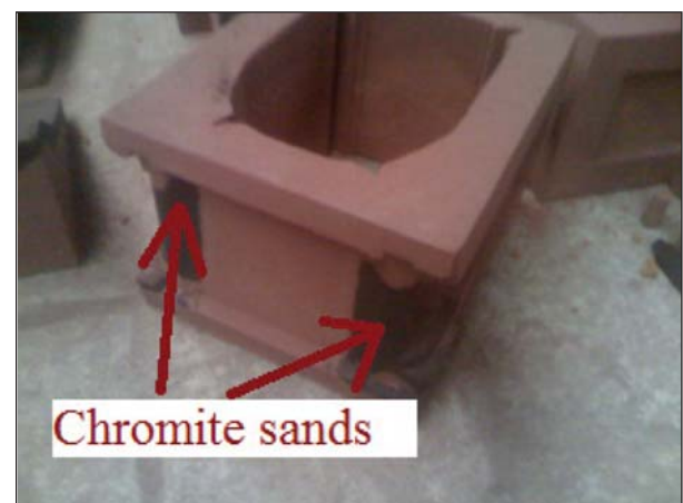
Fig.16: Chromite sands at corners.
