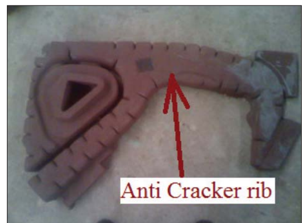
Fig.15: Anti-cracker ribs to arrest hot tear.
