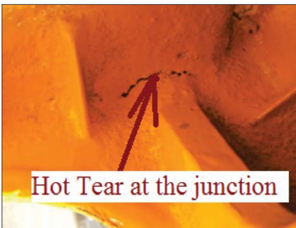
Fig.3: Hot tear defects at junctions.
