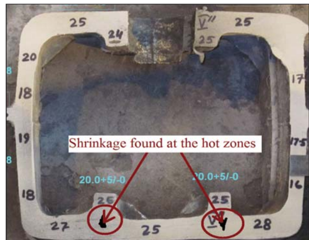
Fig.22: Shrinkage found at the junction.
