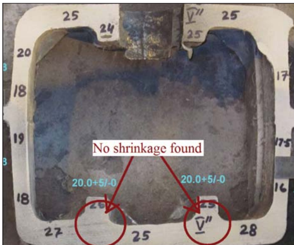
Fig.23: After modification and positioning 4 nos. round risers no shrinkage found at this area.
