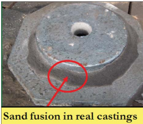
Fig. 19: Sand fusion in real casting
