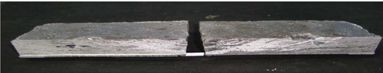
Fig.4: Plate casting with riser \text{\O} 60 \text{ mm} \times 120 \text{ mm} height (S.F 4)
