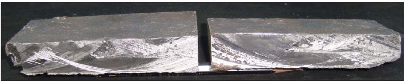
Fig. 6: Plate casting with riser \text{\O} 29 \text{ mm} \times 58 \text{ mm} height (S.F 12)
