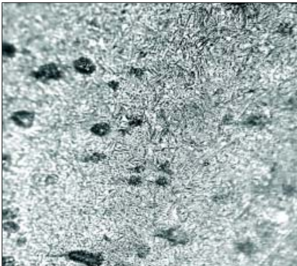
Fig. 1: 0.8% Cu ADI ( austempered at 365°C) etched in 2% Nital and seen at a magnification of 400X.
