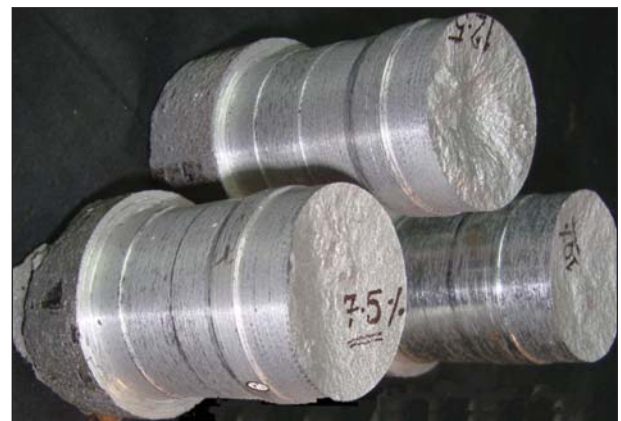
Fig. 1: As cast MMCs Samples Used for Testing of Machinability.
