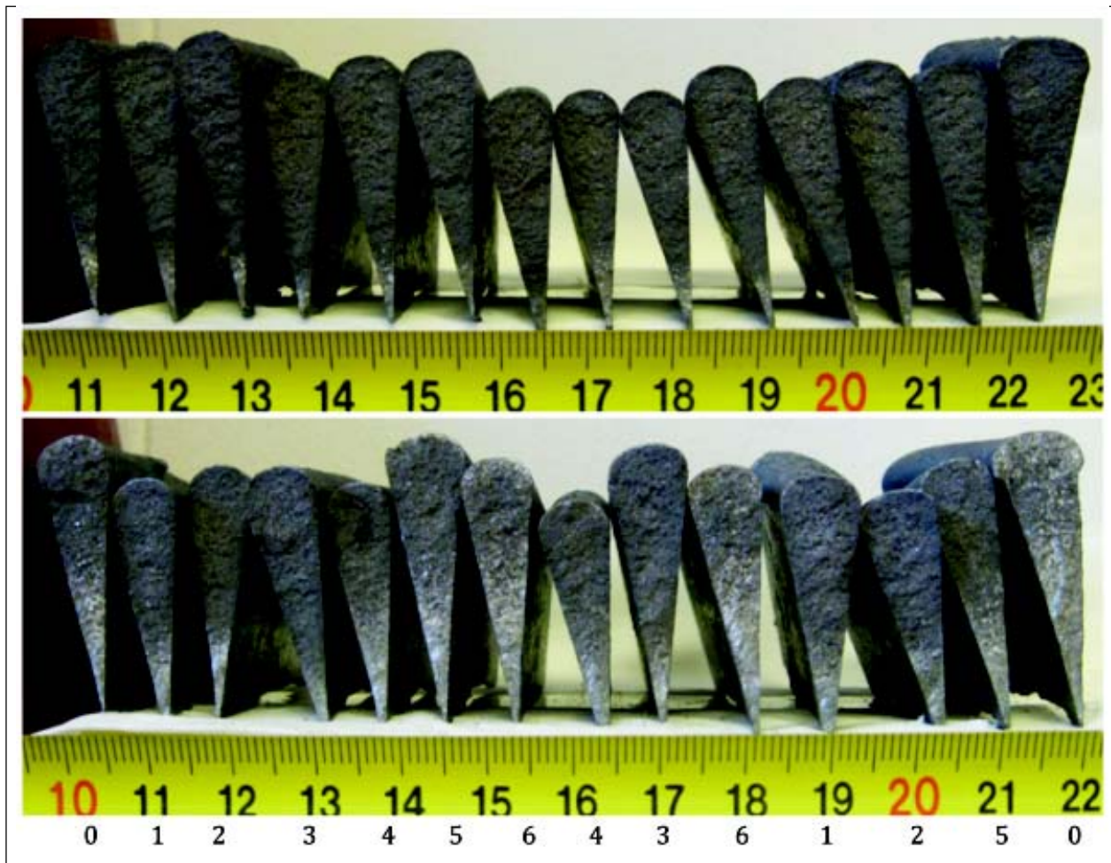
Fig. 7 : Chill wedges from trials without preconditioning for the different inoculants, first and last chill wedge is uninoculated samples. The upper one is the Cr grade while the lower one is the vanadium grade
